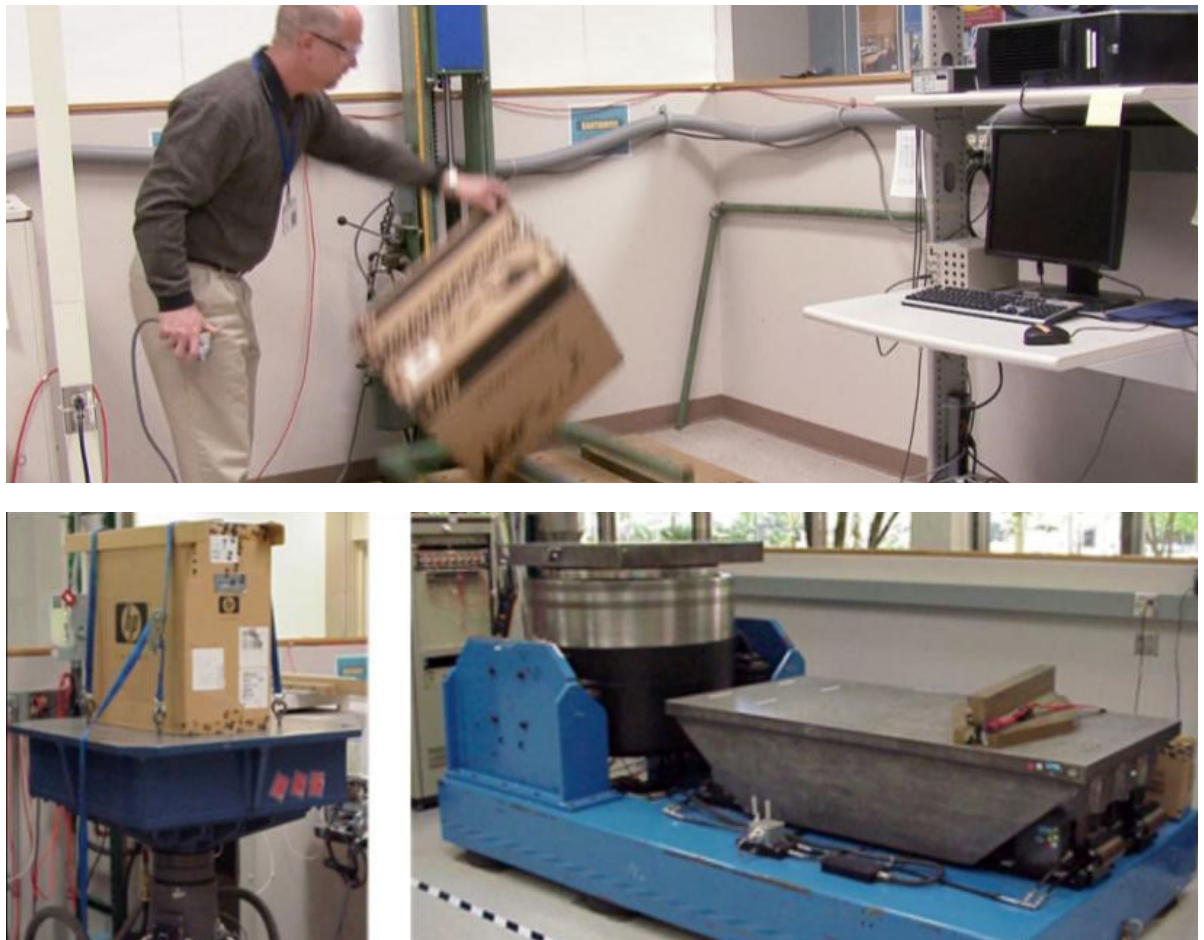
Figure 3. Examples of the tools used to shake and drop our products, simulating real world shipping and usage events
