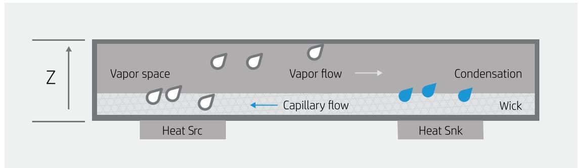
Figure 1. Working principle of a vapor chamber or heat pipe
