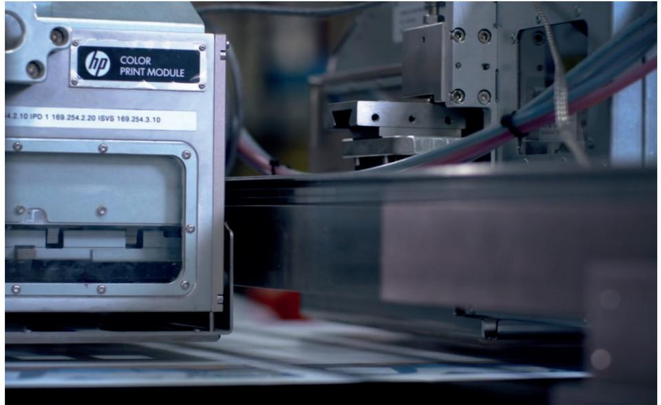
**“The full color CMYK HP C800 Print Module with iDataPrint™ software features automated printhead servicing that manages purging and wiping of the print modules without having the operator manually touch the printheads. The automatic, self-contained cleaning station also eliminates messy and time-consuming start-up and shut-down procedures.”**
