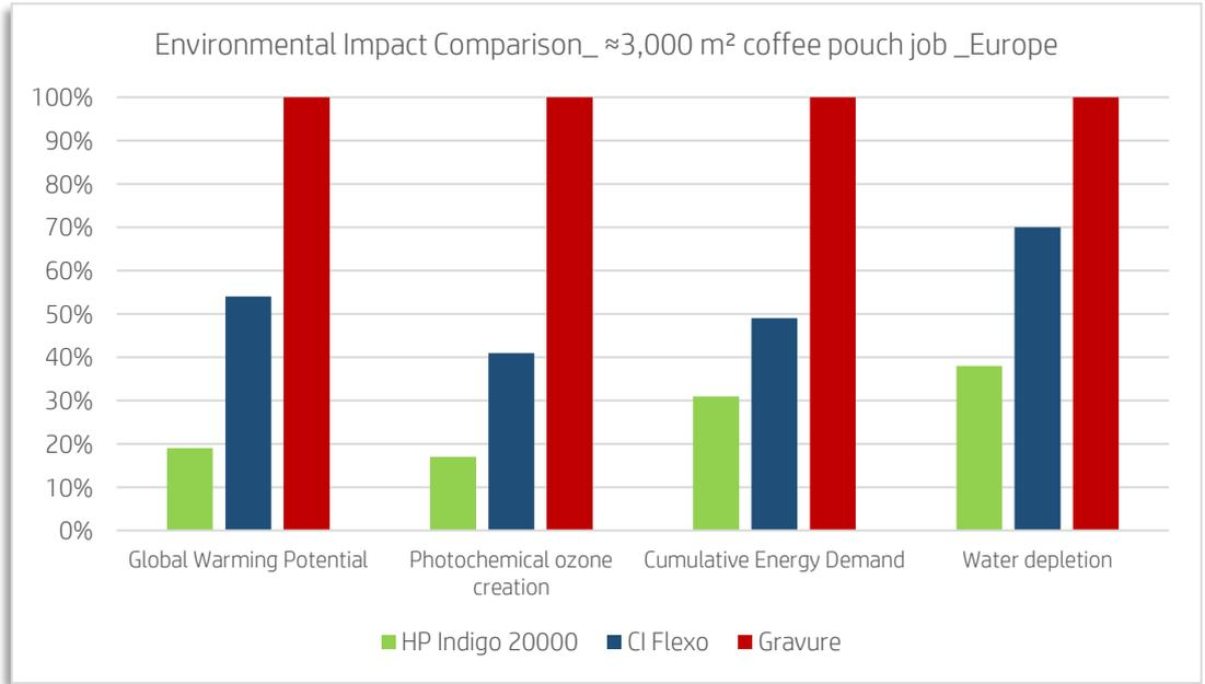
Figure 7.Characterized LCA results for a ≈3,000 m<sup>2</sup> print job using CI Flexo, Rotogravure and HP Indigo 20000 print technologies on a flexible coffee pouch substrate.
