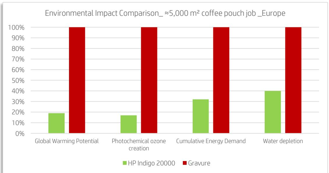
Figure 8. Characterized LCA results for a ≈5,000 m<sup>2</sup> print job using CI Flexo, Rotogravure and HP Indigo 20000 print technologies on a flexible coffee pouch substrate.
