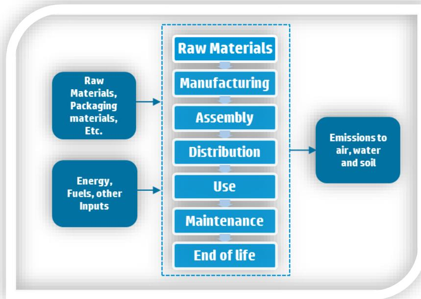
Figure 1. “Cradle to grave analysis” (LCA) process chart
