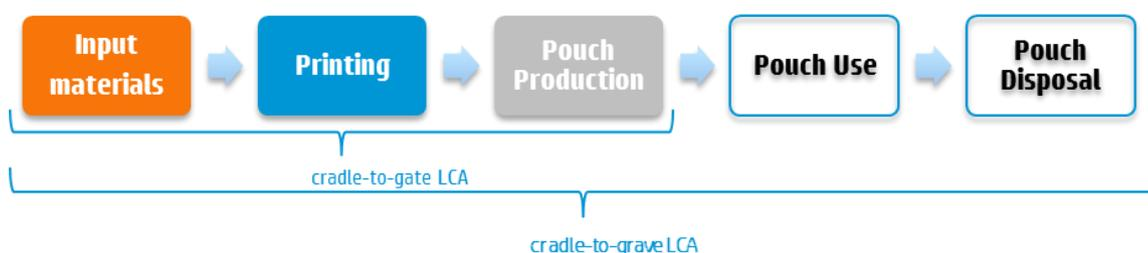
Figure 4. Difference between cradle-to-gate LCA and cradle-to-grave LCA
