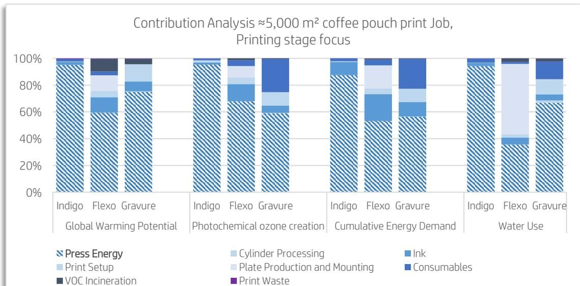
Figure 6. Contribution analysis focus on printing of the characterized LCA results for a  $\approx 5,000 \text{ m}^2$  print job using 3 different print technologies on a flexible coffee pouch substrate.
