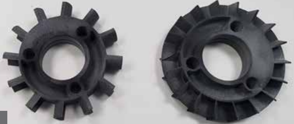
Rotors redesigned and 3D printed with HP Multi Jet Fusion technology
