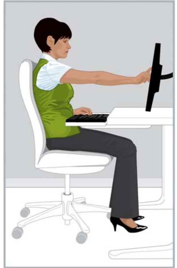
WRONG Touching with an extended arm can quickly tire the shoulder and arm.
