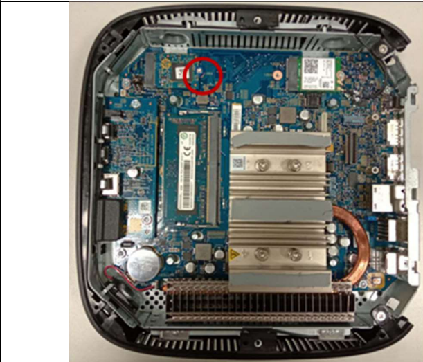
Release 1 pc screw to remove SSD
