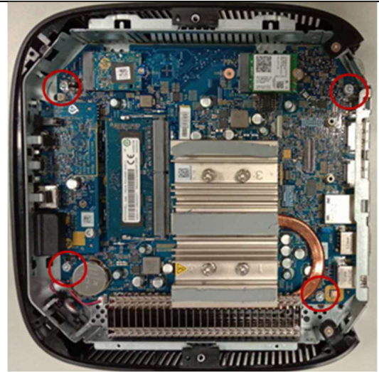
Release 4 pcs screw to remove mother board
